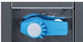
External tank draining system with manual closing and opening mechanism so that operators do not touch the water of the tanks.
